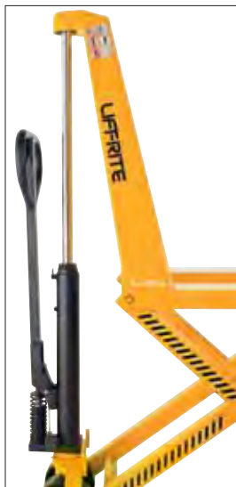
Single-stage cylinder minimizes the risk of leakage. The manual scissor lift truck is fitted with Quick Lift, and can lift 32 mm per stroke of the pump.
