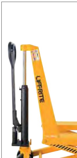
Single-stage cylinder minimizes the risk of leakage. The manual scissor lift truck is fitted with Quick Lift, and can lift 32 mm per stroke of the pump.
